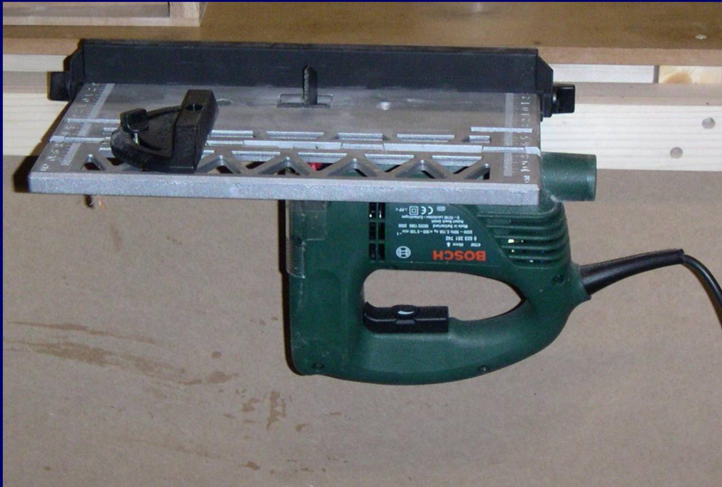
(Ceramic tile-cutter blade to cut fibreglass.)
